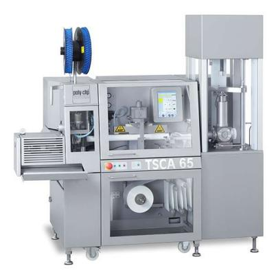
The TSCA 65 D with HDP 40 (hydraulic dosing pump) from Poly-clip System is suitable for all pasty materials such as adhesives and sealants, dental and dowel compounds or 2-component products.
