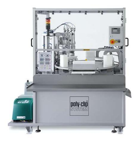
The CBS 15 from Poly-clip System reliably produces very small packs with dosing caps from 50 ml and in the average range from 26.5 to 50 mm.
